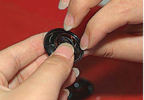
Compression driver assembly. Don't try this at home.
