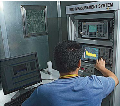
Outside the Electromagnetic chamber in our Testing Laboratories at BEHRINGER City. This is where we test all BEHRINGER products for compliance with standards such as FCC emissions, CE and safety. The facility represents a million dollar investment in Standards Compliance. And includes at least one machine that goes “ping”.
