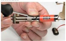
13. Install the preamp to the middle strings behind the bridge by pinching both strings slightly inwards and connecting the clip to them.
