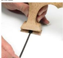
$9.\,\mathrm{Tighten}$  the strings to hold the pickup assembly in place.
