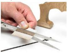
6. Place the spacers on the tape at both side of the pickup.
