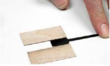
7. Make the spacers the size of the pickup by cutting the excess veneer away.
