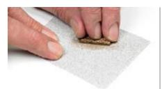
10. Installation of the bridge pickups can be done now. Install the bridge pickups to the wing slots by using two of the cork pieces supplied. You may need to adjust the cork thickness by sanding it. The pickup and the cork should fit somewhat tight (but not to tight!), to avoid any disturbing resonance. If thicker cork is needed, fashion shims from, for example, a wine cork.
