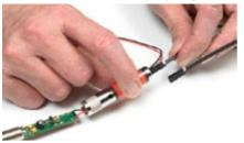
Connect the plastic connector of the body pickup, with the holes at the plastic connector facing up, to the lower set of pin headers at the circuit board.
