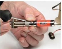
By turning the screw clockwise there is more of the body pickup. By turning the screw counter-clockwise, more of the bridge pickup will be heard.
