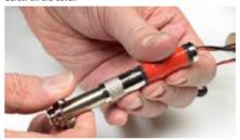
NOTE! There is a small hole at the cover's side. This is an access hole to the blend control at the circuit board. Make sure that you tighten the cover enough so the hole is directly over the blend control.
