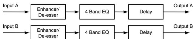
This is a dual-mono channel strip. It provides enhancer/de-esser, EQ, and delay.
