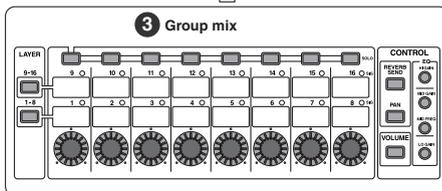
The sources 1–40 being input via REAC are mixed by the M-48's 40-channel mixer. Settings and operation of the 40-channel mixer are shared between the mixing engineer and the musician.
