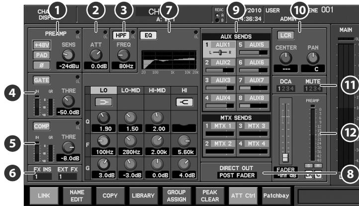
The principal operations for an input channel can be performed in the CHANNEL DISPLAY screen.
