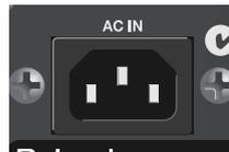
Connect the included power cord to the AC INPUT connector.
