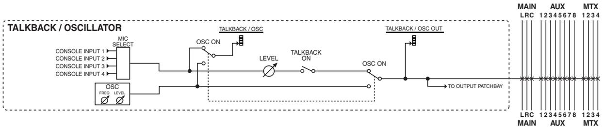
Talkback is a function that sends the input of a mic connected to the CONSOLE IN1–4 on the rear panel jack to an AUX, MTX, MAIN L/R/C, or the output patchbay. This is useful when the mixer operator needs to convey instructions to performers on stage or to staff.
