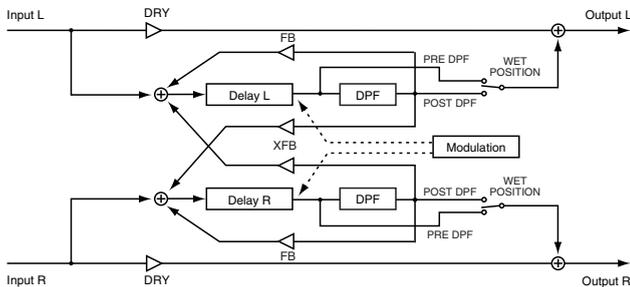
This is a stereo-in, stereo-out cross-modulation delay.
