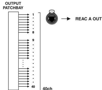
When the M-300's REAC is set to MONITOR/BROADCAST (p. 140), the REAC A port operates as the REAC split. In this case, the M-300 cannot output signals to the REAC A.
