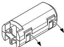
2. Attach a ferrite core near the RJ45 plug on the Ethernet cable.
