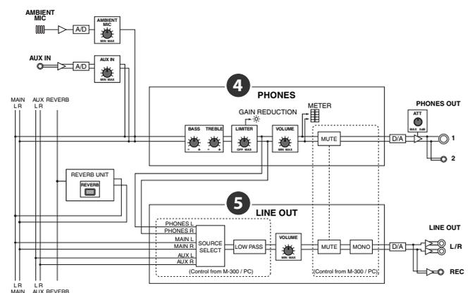
The M-48 provides two sets of output: PHONES and LINE OUT.
