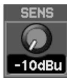
Knobs in the screen can be operated by the knobs of the CHANNEL EDIT section or by the value dial. To use the value dial, move the cursor to the desired knob.
