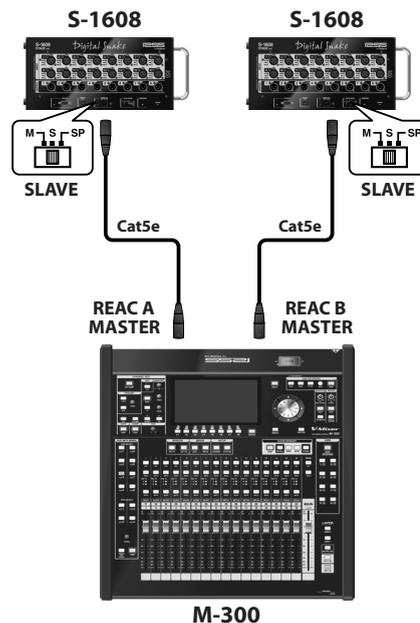
The default input/output patching between the M-300 and input/output units connected to REAC ports A/B is as follows:
