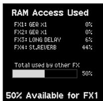
This area indicates the amount of RAM access used for each of the currently operating FXs. You can also check the amount of RAM access available for the selected FX.
