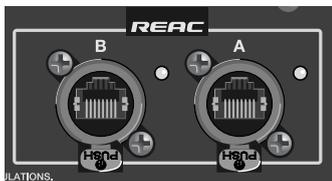
These are RJ45 connectors for connecting input/output units such as the S-1608, S-0816, or S-4000S via Cat5e Ethernet cables.
