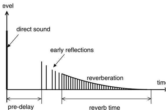
The reflected sounds reach the listener in the following order. The pre-delay is the time from when the direct sound is heard until the reverb arrives. The reverb time is the duration until the reverb disappears.
