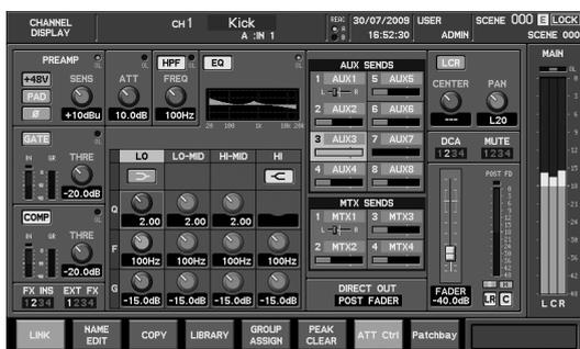
This area shows mixer parameters, system settings, and meters. You can use the CHANNEL EDIT section, the function button section, and the screen controller section to perform operations in the display.
