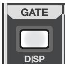
In this area you can operate the gate/expander that is provided for CH1–32.
