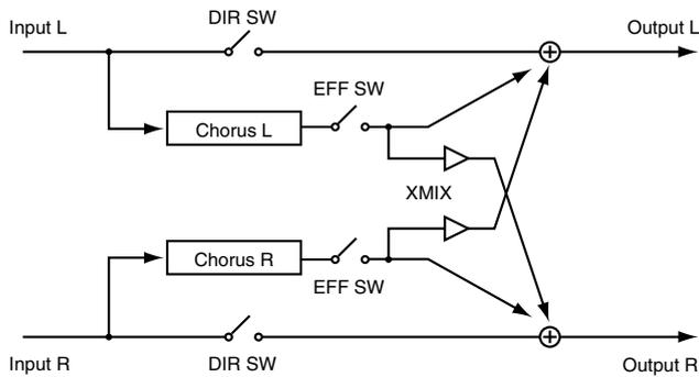
This is a stereo-in, stereo-out chorus. It lets you apply chorus without impairing the position of the sound image that's been set for the stereo input, by panning or other means.
