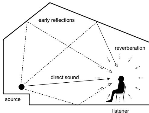
The sound you normally hear is divided into three types: “direct sound,” “early reflections,” and “reverberation.” The “direct sound” is the sound that reaches the listener directly from the source. “Early reflections” are sounds that have reflected one to several times from the walls or other surfaces of the room. “Reverberation” is sound that has reflected many times before reaching the listener.
