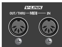
These connectors are for connection with MIDI equipment. An IN connector (for reception) and an OUT/THRU connector (for transmission and "thru") are provided. You can use the REMOTE popup to switch between the OUT and THRU functions.
