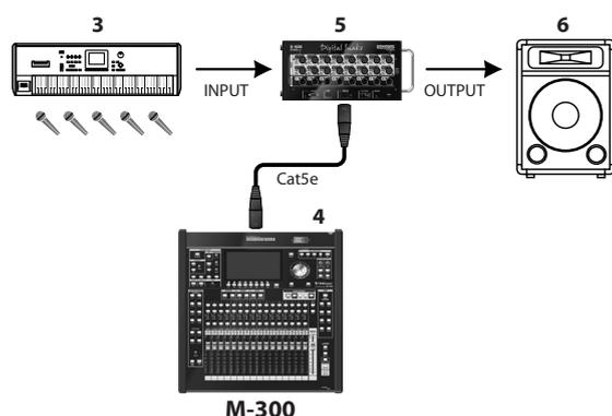
1. Connect your input/output units (S-1608, S-0816, S-4000S, etc.) to the M-300's REAC port.
