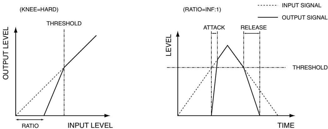
A ducking applies a user-adjustable level of attenuation (RANGE) to input signals that are higher than the threshold level.
