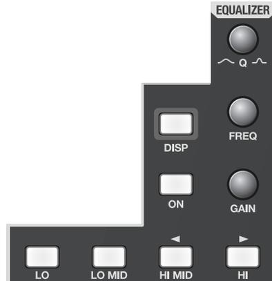
In this area you can operate the 4-band EQ or 8-band EQ that is provided on each channel.
