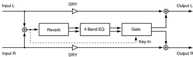
This is a mono-in, stereo-out reverb. It provides a gate that can be used for gating or ducking, allowing you to cut the reverb during its decay, or to cut the reverb when the level of the original sound is high.
