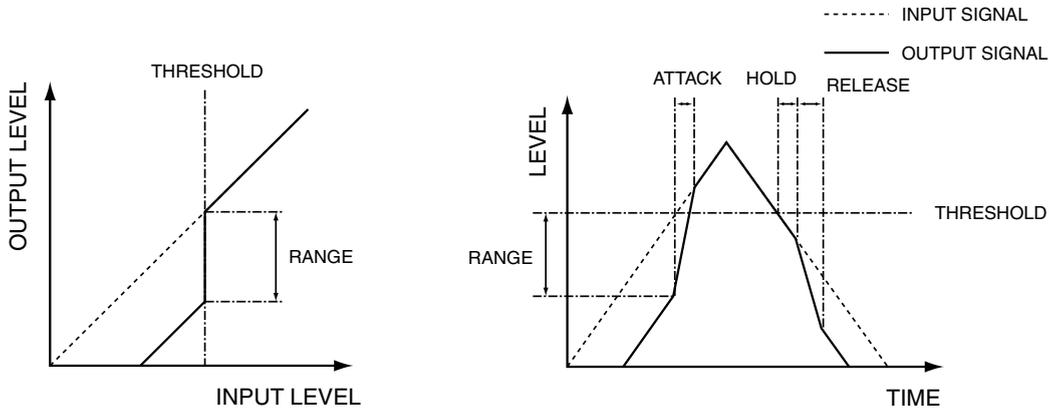
An expander applies a user-adjustable ratio of attenuation (RATIO) to input signals that are lower than the threshold level.
