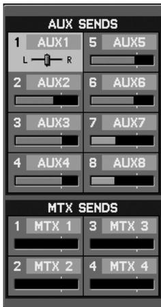
Here you can adjust the sends from the channel to the AUX1–8 or MTX1–4 buses.
