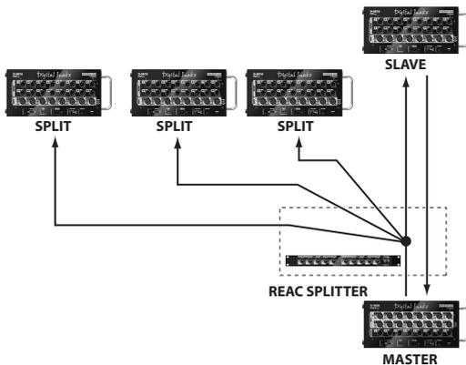
To assign a REAC device to operate in split mode, you must set its REAC mode to Split. The REAC split device will function solely to receive signals from the REAC master device.
