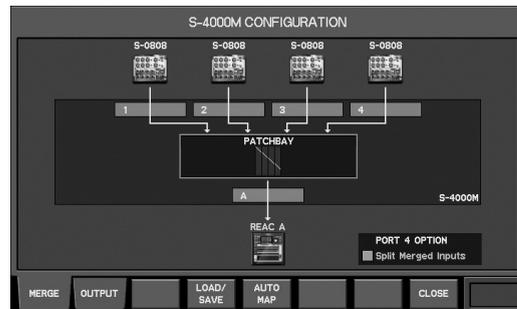
If the "Split Inputs to PORT4" button in the PORT4 OPTION is checked, then the S-4000M's split function is already turned on. The following steps will not be necessary.
