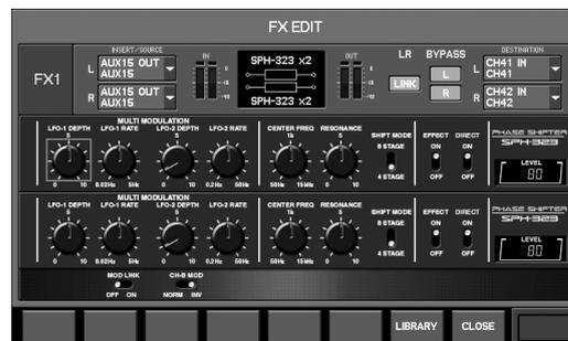
This is a phase shifter that models the Roland SPH-323 Phase Shifter. The original was mono-in, mono-out, but this modeling is a dual-mono design with two units in parallel. The MOD LINK Sw allows you to use this as a stereo-in, stereo-out effect.
