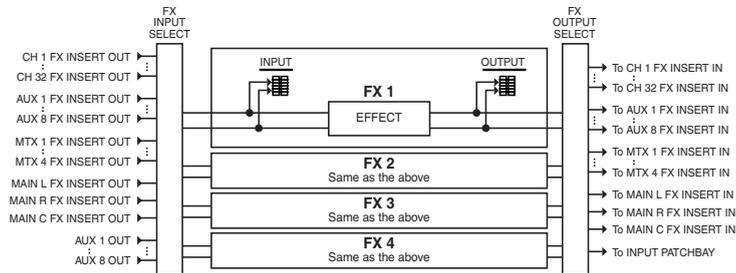
The M-300 contains four internal effects (FX1–FX4), each of which allows you to select from 11 different effect types including reverb, delay, and 31-band GEQ.
