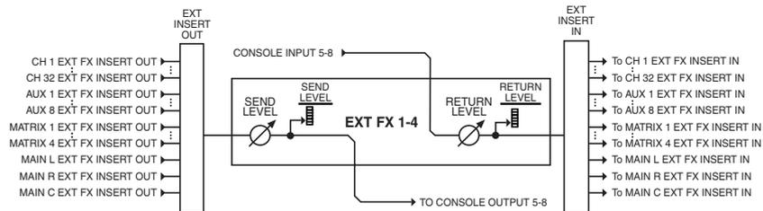
You can use the CONSOLE IN 5–8 and CONSOLE OUT 5–8 jacks located on the M-300's rear panel to insert up to four external effects devices into channels. The four external effects devices are shown virtually as an EXT FX1–EXT FX4 rack, allowing you to adjust the input levels and insert them into channels.
