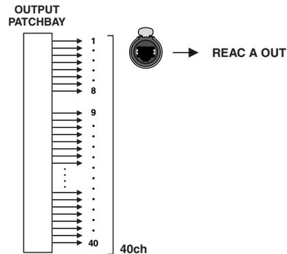
When the M-300's REAC is set to MONITOR/BROADCAST (p. 140), the REAC A port operates as the REAC split. In this case, the M-300 cannot output signals to the REAC A.
