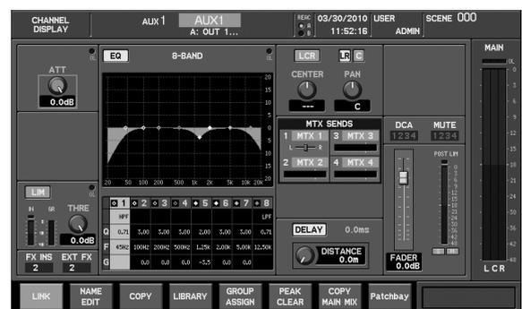
Even if you operate the knobs of the CHANNEL EDIT section without accessing the CHANNEL DISPLAY screen, the value of the currently-operated parameter is shown in the sub-display area.
