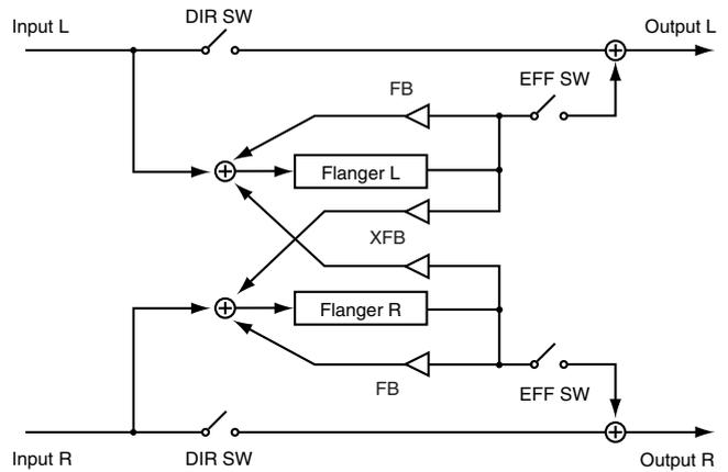
This is a stereo-in, stereo-out flanger. It lets you apply flanging without impairing the position of the sound image that's been set for the stereo input, by panning or other means.
