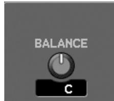
This adjusts the left/right output balance sent from MAIN L/R or stereo-linked AUX/MTX in a range of L63–R63.
