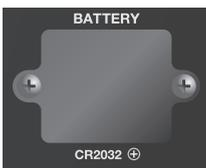
This slot contains a lithium battery that maintains the M-300's clock function and preserves the mixer settings.
