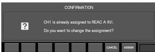
If an input port is already patched to the channel, a message will ask you to confirm the input patching change.
