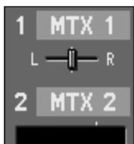
If the send-destination is a stereo-linked pair of MTX, this slider adjusts the left/right position in a range of L63–R63. This is shown for the odd-numbered MTX send.
