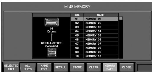
In this tab you can manipulate the memories of the M-48 unit that is selected in the M-48 list.
