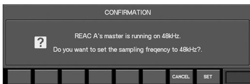
This confirmation message will appear if there is a difference in sampling frequency between the FOH console (master) and the MONITOR/BROADCAST console (split).
