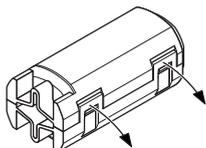
2. Attach a ferrite core near the RJ45 plug on the Ethernet cable.
