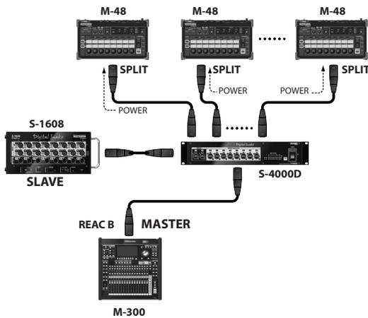
Use the REAC B port to connect M-48 units to the M-300. A separately available S-4000D splitter and power distributor is required in order to connect M-48 units.
