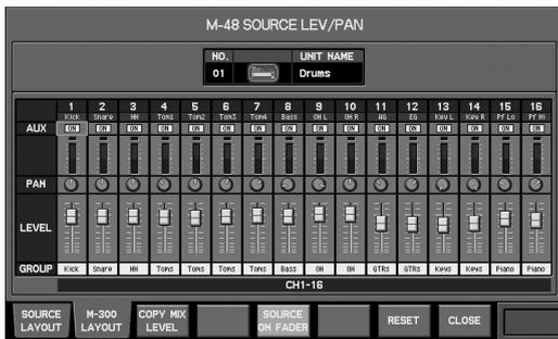
This shows the sources as they are seen from the M-300's fader module section. This display will change according to the M-300's channel layer.
