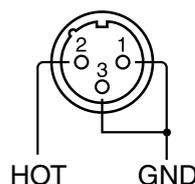
INPUT jacks provide phantom power (+48V/14mA).
