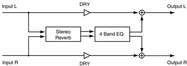
This is a stereo-in, stereo-out reverb. It adds reverberation without impairing the position of the sound image that's been set for the stereo input, by panning or other means.
