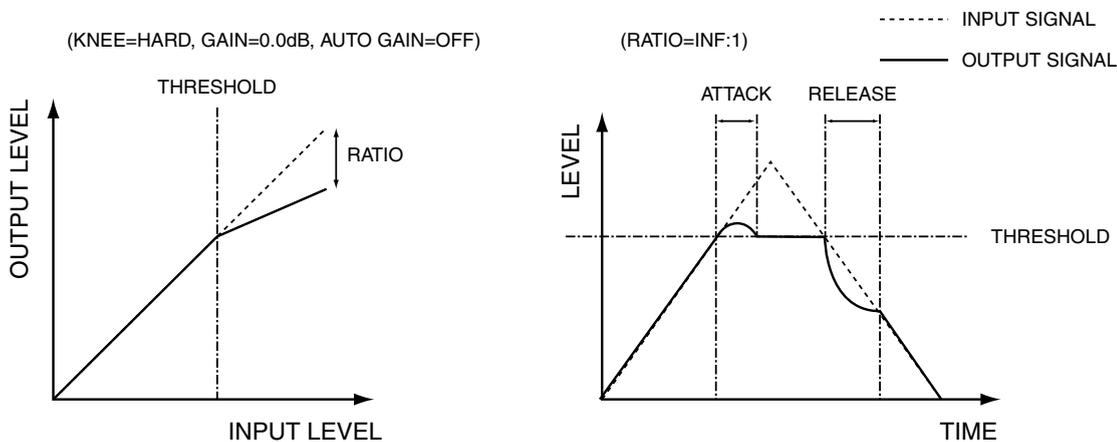
The COMPRESSOR popup is used to perform compressor operations.
