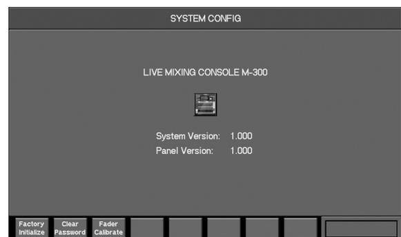
The M-300 will start up in SYSTEM CONFIG MODE, and the SYSTEM CONFIG screen will appear.
