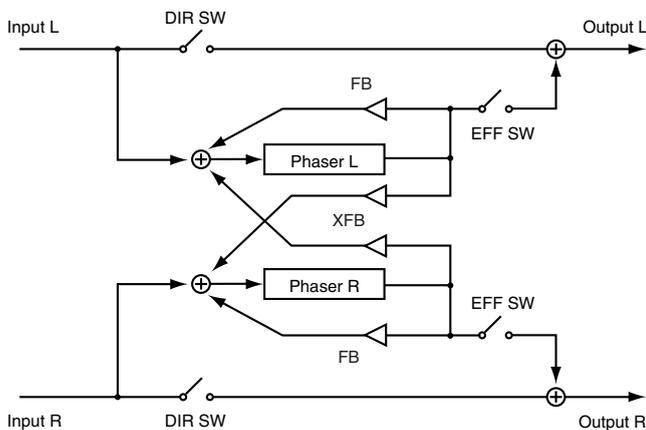
This is a stereo-in, stereo-out phaser. It lets you apply a phaser effect without impairing the position of the sound image that's been set for the stereo input, by panning or other means.
