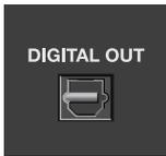
This is optical type jack that outputs a consumer format (IEC-60958 compliant) digital audio signal. By default, MONITOR L/R is patched to these jacks.
