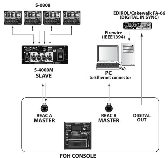
The M-300's REAC port connected to a PC must be a REAC master.
