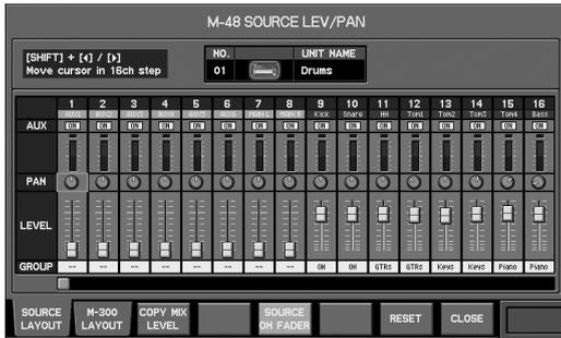
This shows the sources arranged in order of their number (the order in the M-300's REAC B output patchbay).
