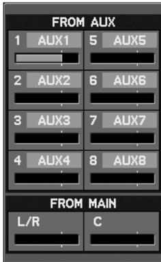
These adjust the send levels from the AUX or MAIN to the MTX. The FROM AUX send /FROM MAIN send are structured as follows:
