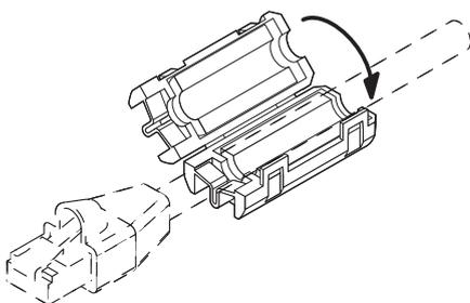
4. Connect the plug with the ferrite core to the M-300's REAC port.
