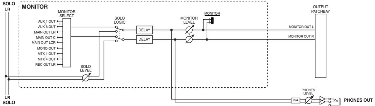
Monitoring is a function by which the AUX, MTX, MAIN, or USB memory recorder signal that you select as the monitor source can be sent from the output jacks or headphone jack. This is used mainly by a mixing engineer to monitor the signals.
