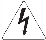
This symbol is intended to alert the user to the presence of uninsulated "dangerous voltage" within the product's enclosure that may be of sufficient magnitude to constitute a risk of electric shock to persons.
